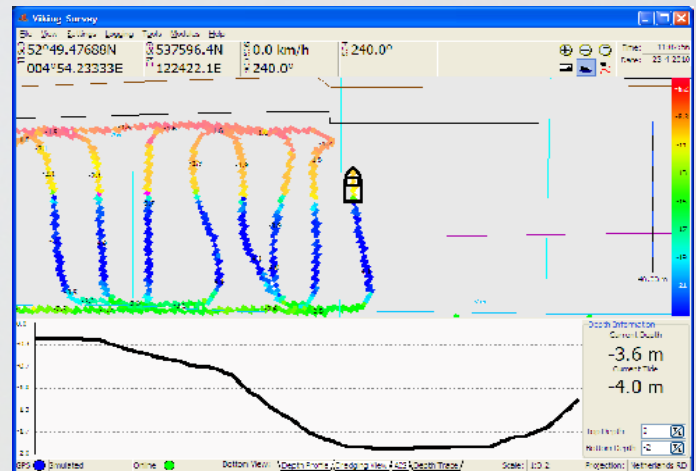
Viking Survey used during a single beam survey
