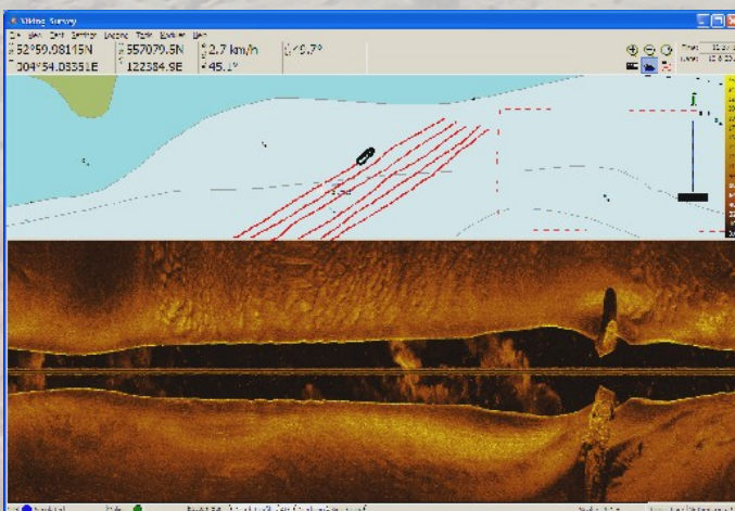
Sidescan Survey of a large wreck in the Waddenzee
